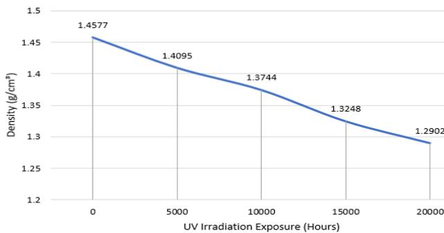
**Fig. 4:** Density (g/cm<sup>3</sup>) versus UV exposure (hours)
