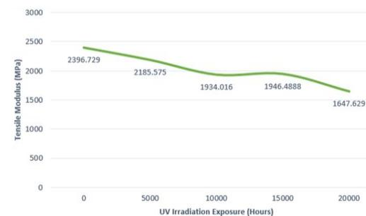
Fig. 4: Tensile modulus (MPa) versus UV (hours)
