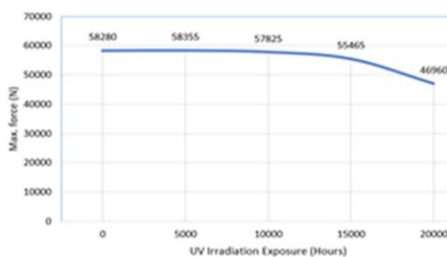
Fig. 1: Maximum force (N) vs UV exposure (hours)
