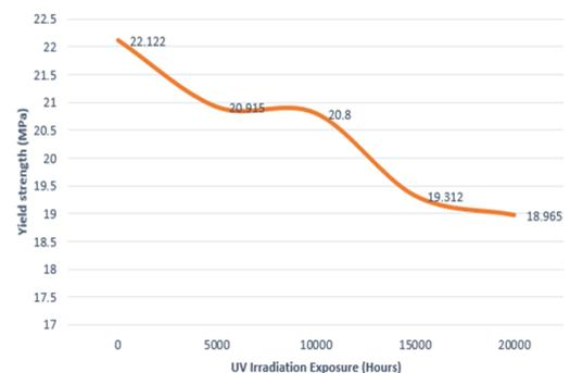
Fig. 3: Yield strength (MPa) versus UV (hours)
