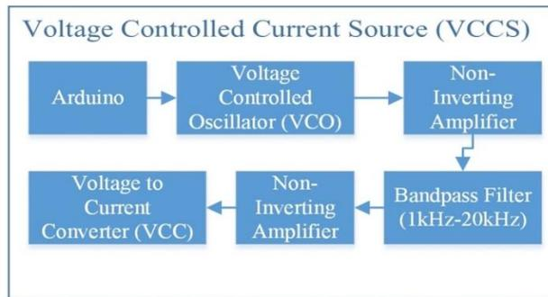
**Fig. 2:** Voltage Controlled Current Source (VCCS) Circuit Design.
