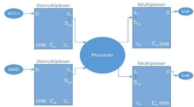
**Fig. 3:** Multiplexer/Demultiplexer Design for High-Speed EIT System.
