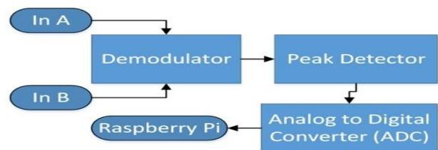
**Fig. 4:** Voltage Measurement Diagram.
