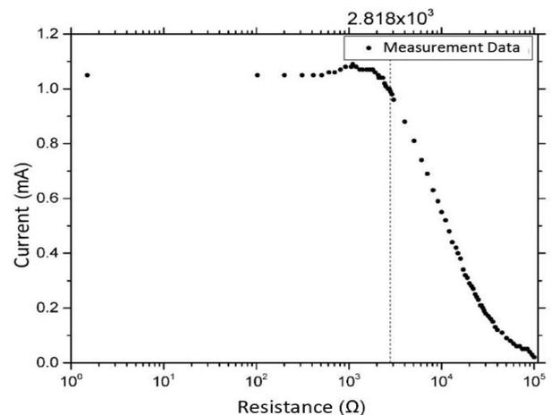
Fig. 8: VCCS Load Ranging from 1 – 100 K $\Omega$  That Used to Conduct Test the Ability of EIT for Supporting High Impedance Tissue.
