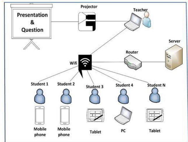
Fig. 1: Standard architecture of mobile-based CRS.
