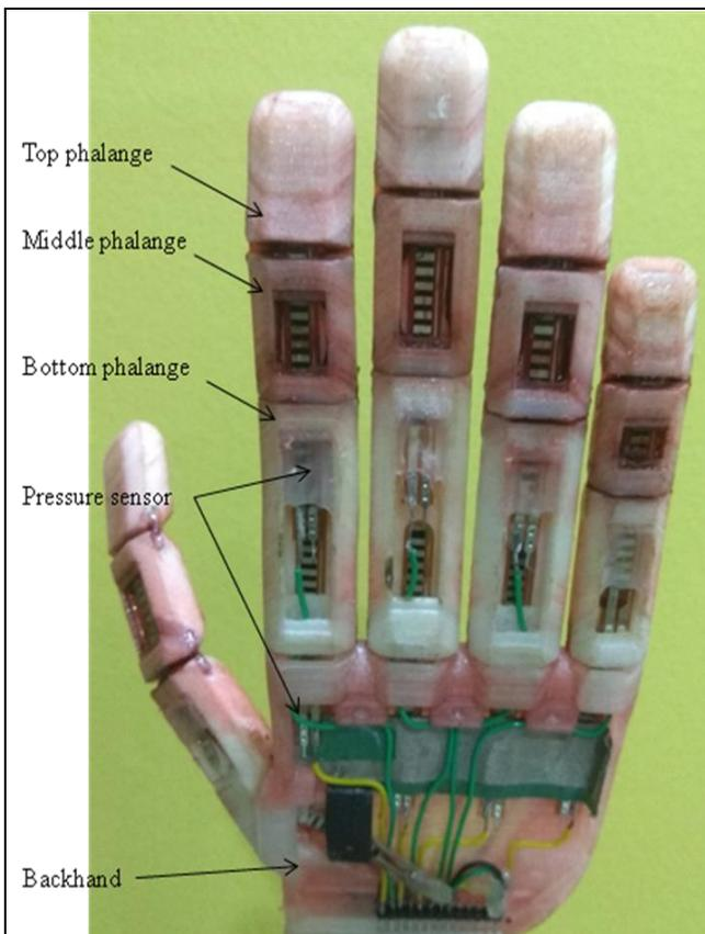
Fig. 12: Slave prototype backhand view.
