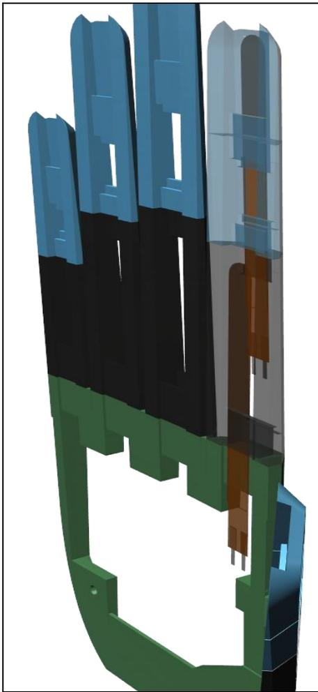
**Fig. 3:** Perspective view of the master components or glove design to emphasise the sensors placement.
