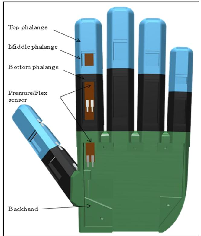
**Fig. 5:** Backhand view of the slave components or hand design.
