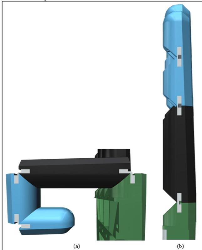
Fig. 8: Robotic hand in (a) curling position and (b) straighten position.
