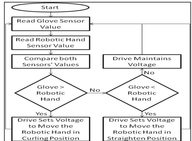
Fig. 9: Pressure sensors comparator system flowchart.
