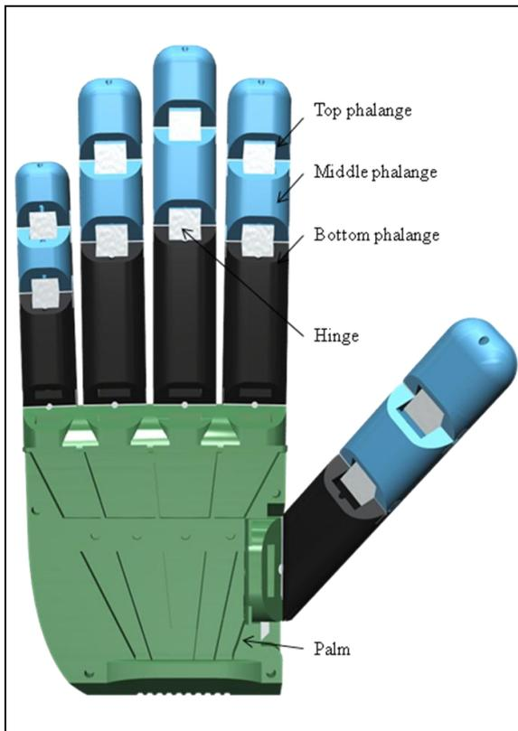
**Fig. 4:** Palm view of the slave components or hand design.
