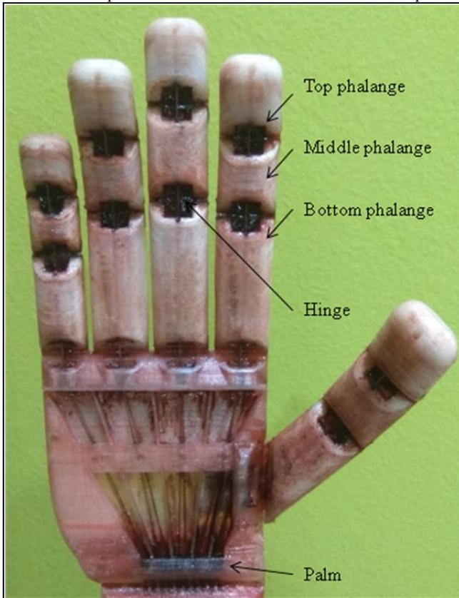
Fig. 11: Slave prototype palm view.
