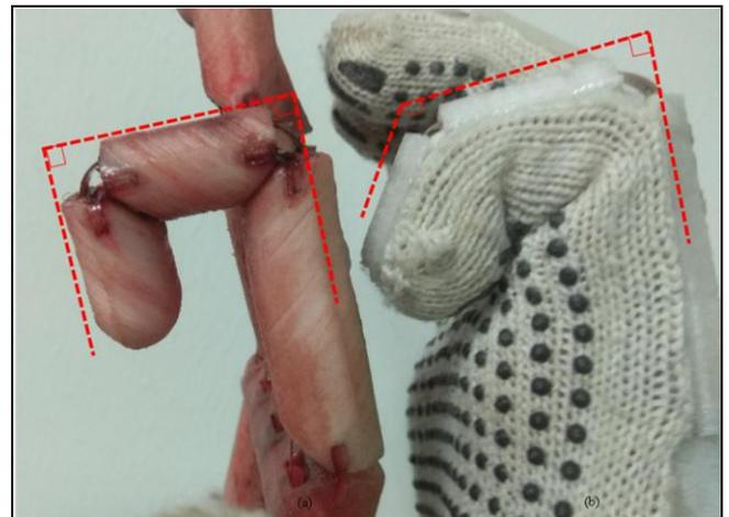
Fig. 14: The (a) slave prototype and (b) master prototype demonstrate a hooking gesture through the index finger. The red dashes lines indicate the angular positions.
