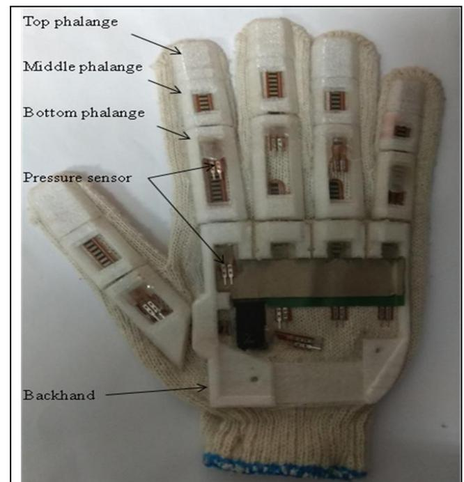
Fig. 10: Master prototype components.
