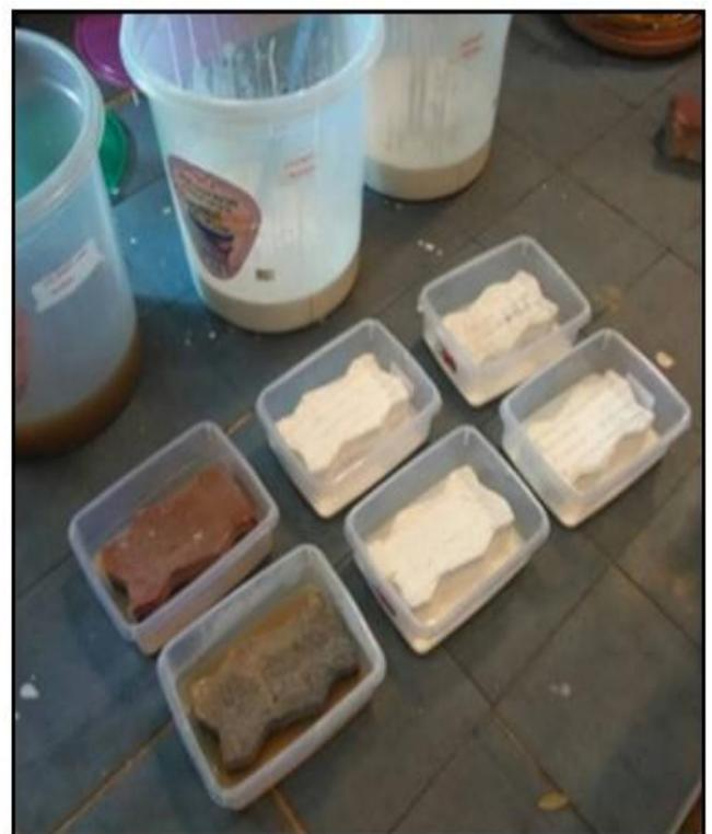
Fig. 4: Pavers were submerged in coatings in immersed method.
