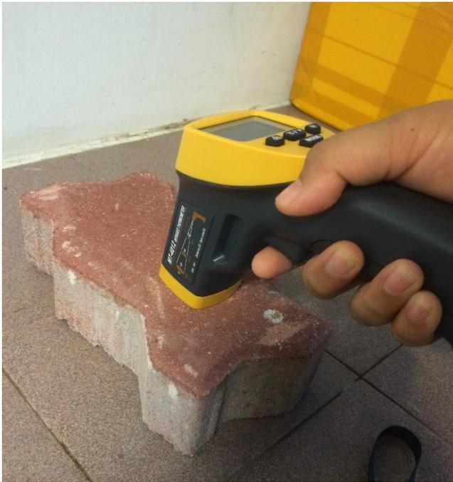
Fig. 5: Surface temperature recorded by using LCD Laser Infrared Digital Temperature Thermometer Gun.
