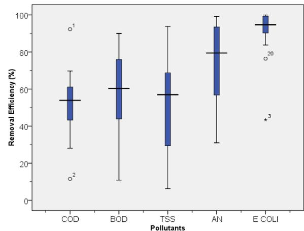
Fig. 9: Removal Efficiency for Klang RWTP
