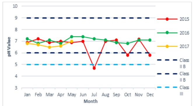
**Fig. 2:** Trend in pH data at RWTP outlet point from Jan 2015 to May 2016
