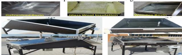
Fig. 2 Different views of the first designed solar stil
