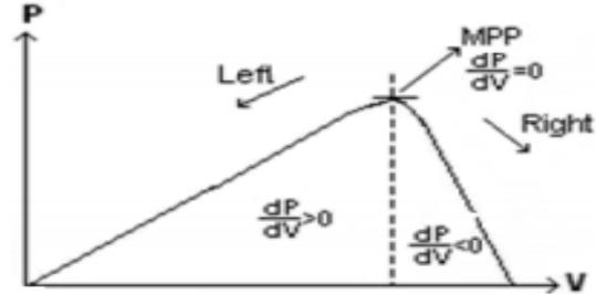
Fig-6: P-V curve of solar module with IC method
