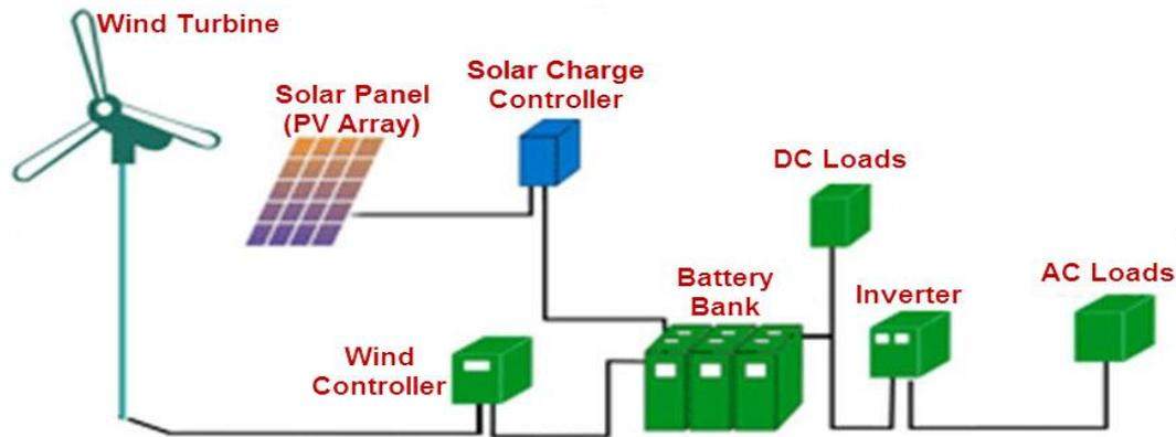
Figure.3: wind-solar system
