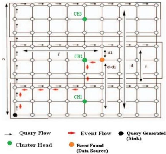
Figure 4.: Cluster based comb needle model
