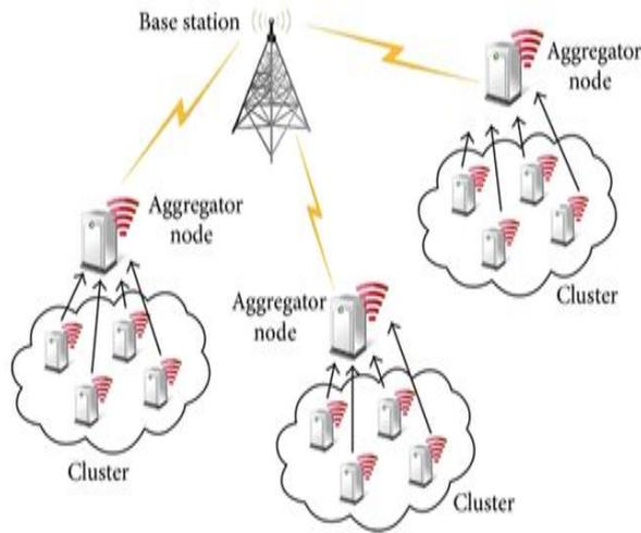
Figure 1: Data aggregation in WSN
