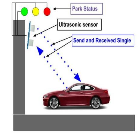
Figure 2.: Ultrasonic Sensor Work
