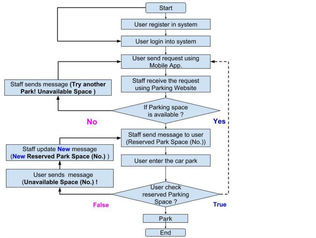
Figure 12.: Algorithm of System Operations.
