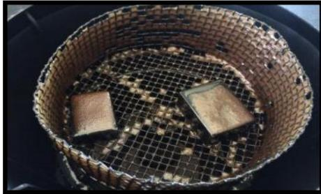
Fig. 8: Quenching in Oil Medium
