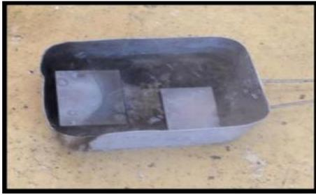
Fig. 7: Quenching in Sea Water Medium
