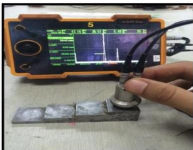
Fig. 9: Calibrate the Probe Process
