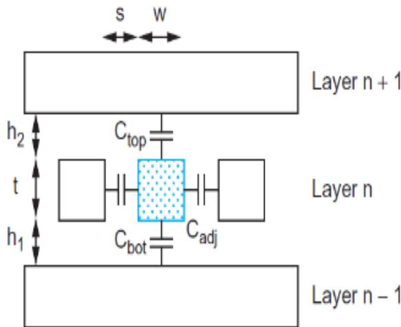
Fig.2: Total Capacitance of the conductor.
