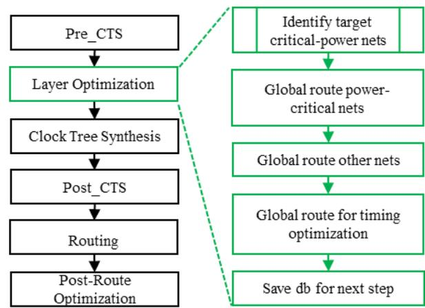
Fig. 4: Baseline design flow vs. featured flow.
