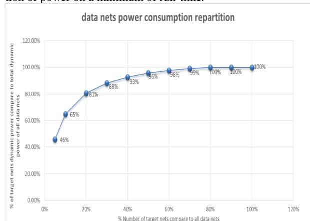
Fig. 5: Data nets dynamic power consumption distribution.
