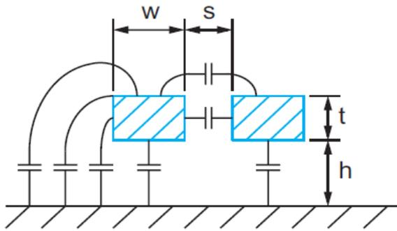
Fig.1: Wire Capacitance
