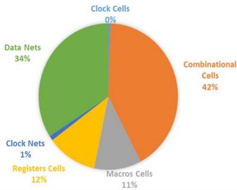
Fig.3: Total power repartition in a digital design block made with 7nm.
