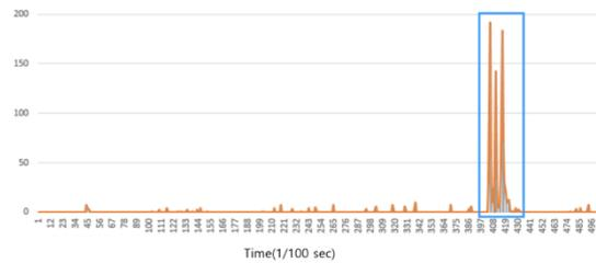
Figure 5: Example of vibration values recognized during shooting moment
