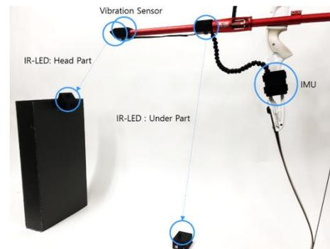
**Figure 2:** Structural diagram of the screen archery system using a VR shooter
