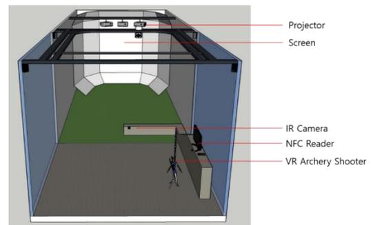
**Figure 1:** Design diagram of the screen archery studio for indoor archery experience
