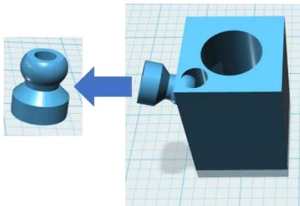
Figure 4: Example of case design to ensure flexibility between connecting lines
