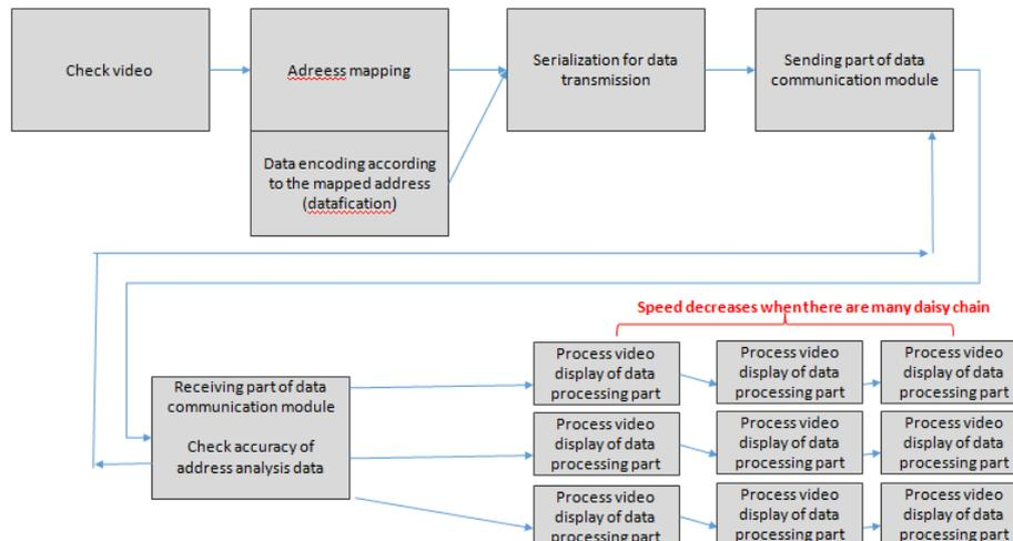
Figure 2: Overall configuration of the control unit
