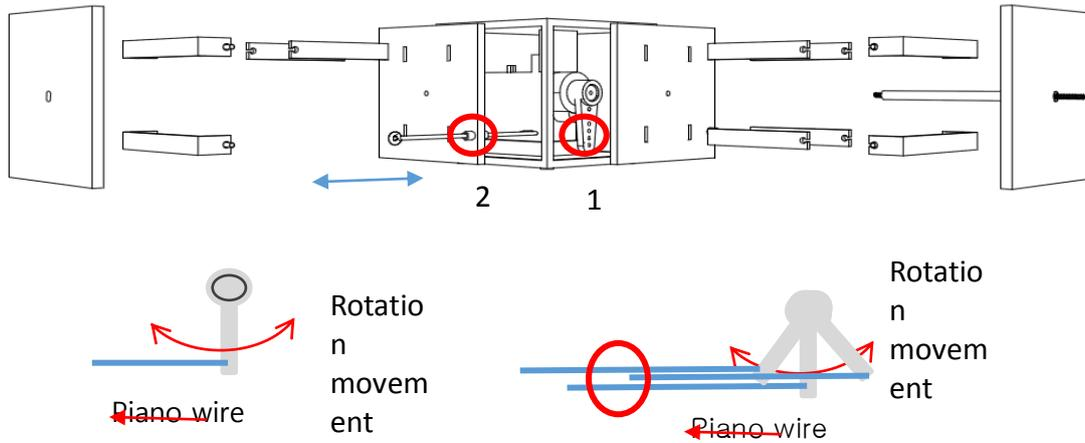
Figure 9: Arm structure and two-way movements
