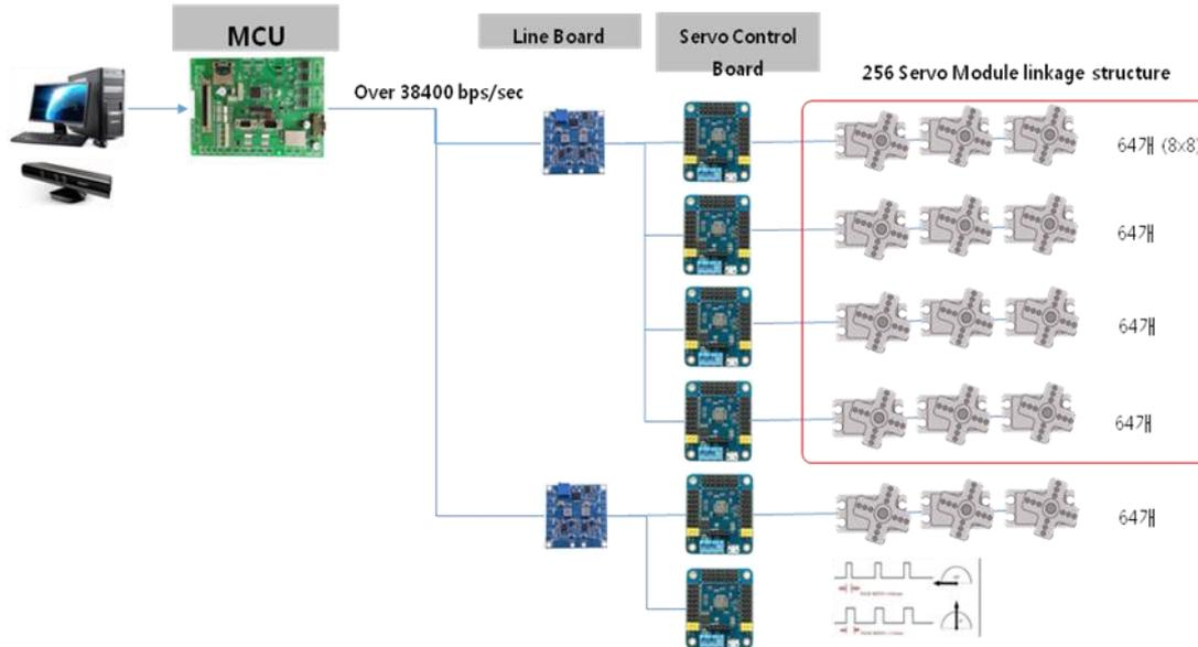
Figure 1: Module linkage Structure
