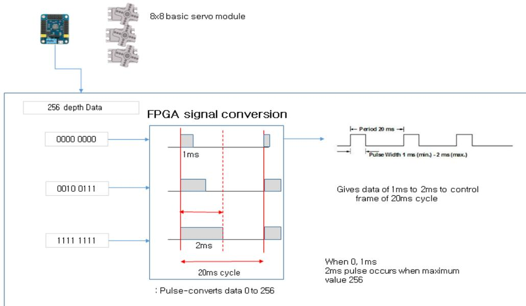
Figure 4: FPGA signal conversion.
