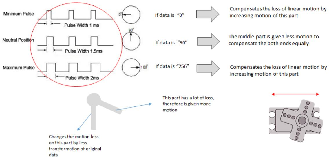
Figure 10: The scope of loss of the motion in accordance with the pulse control signal
