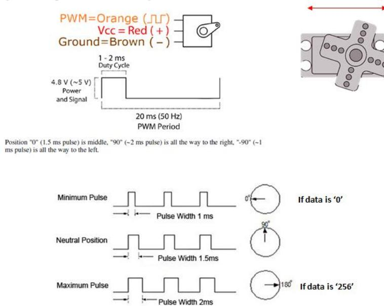
Figure 5: Operation method of servo
