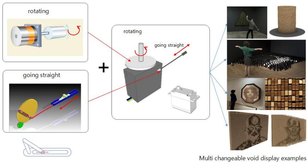
Figure 7: The development of the arm type mechanism
