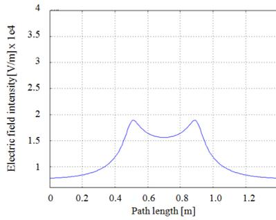
**Figure 1:** In case of Horizontal conductor type, the electric field extraction path and field intensity
