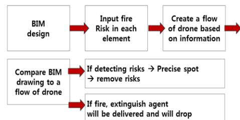
Figure 5: Integration between BIM and Drone
