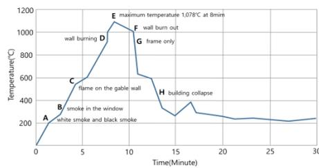
Figure 1: Fire process on wooden structure
