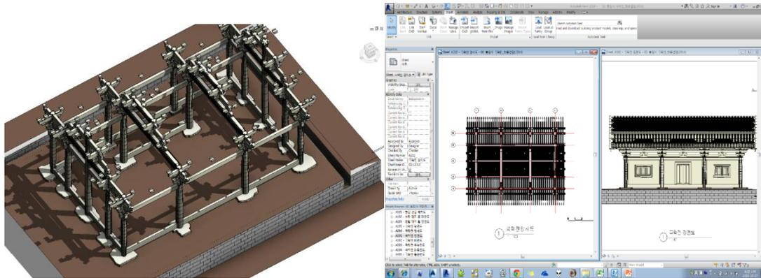
Figure3: BIM generation process in Bongjeongsa
