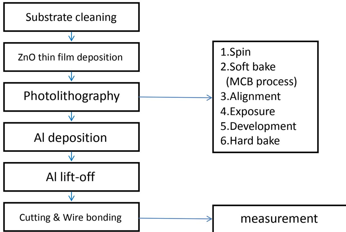
**Figure 1:** Fabrication process chart of ZnO thin film SAW filter
