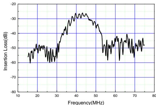
Fig 4: Frequency response of ZnO(20µm)/Al/SiO<sub>2</sub> SAW filter
