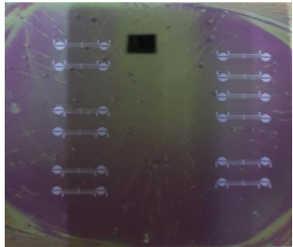
**Figure2:** Fabrication of ZnO thin film SAW filter by Photolithography
