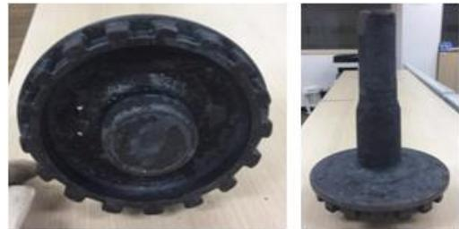
Figure 14: Hot Forging Press mold and Prototype
