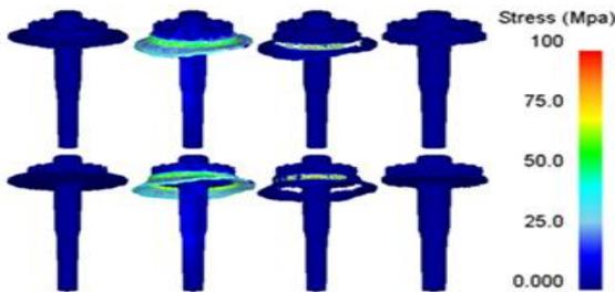
Figure 11: 4<sup>th</sup> Station Hot Forging Stress Analysis Result
