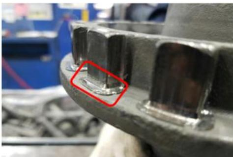
Figure 17: Defects in Cold Forging
