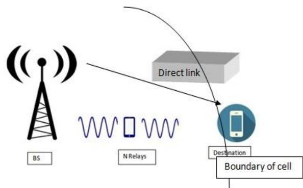
Figure 1: Illustration of a co-operative system.
