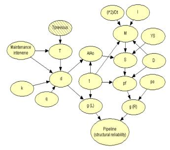
Fig. 3: Structural reliability of pipeline as a DBN.
