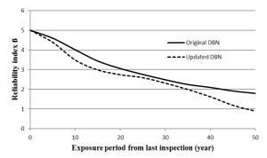
Fig. 4: Predicted reliability of pipeline failure for an exposure period of 50 years.
