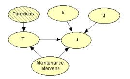
Fig. 2: DBN model of corrosion growth with integration of maintenance variable.
