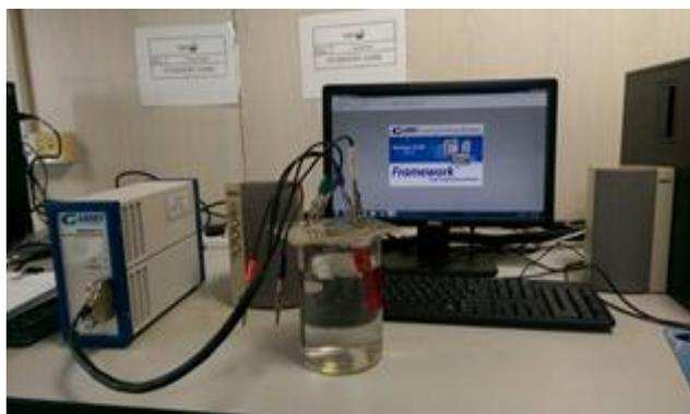
Fig. 1: The setup of Gamry's software instrument for potentiodynamic testing
