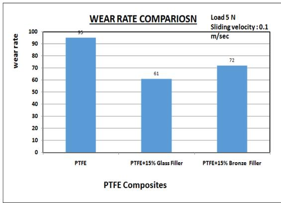
Fig 6: Wear rate of PTFE and PTFE composites
