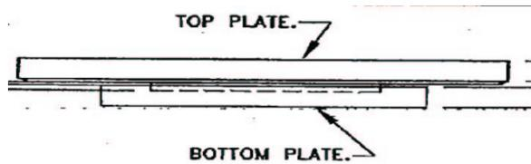
Fig 3:..PTFE Vs SS316 ALIGNMENT
