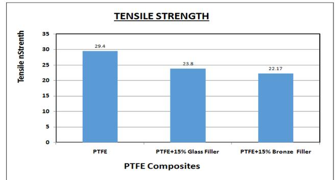
Fig .10: Tensile strength of PTFE and PTFE composites
