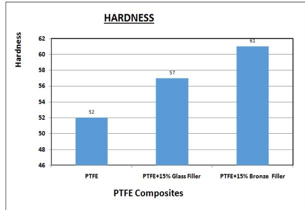
Fig 9: Hardness of PTFE and PTFE Composites
