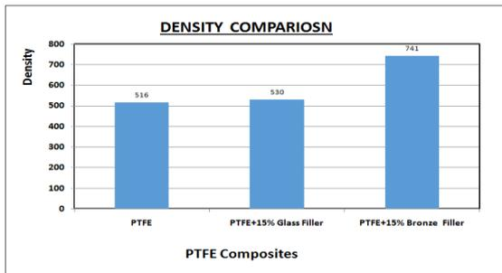
Fig.8: Density of PTFE and PTFE Composite
