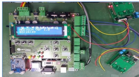
Figure 9: Main control board of LED security light
