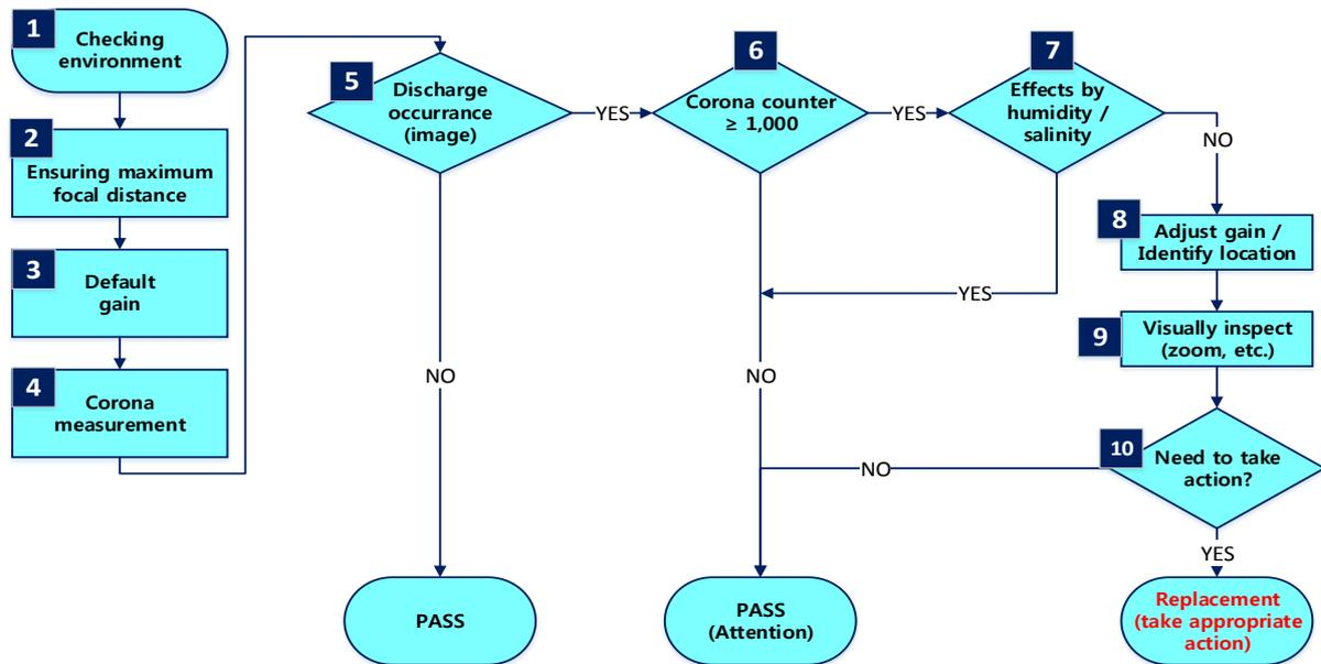
Figure 7: Ultraviolet corona determination criteria (plan)
