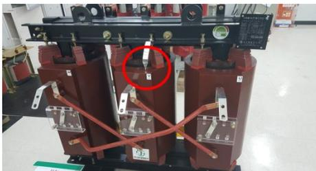
Figure 1: Transformer used for corona measurement
