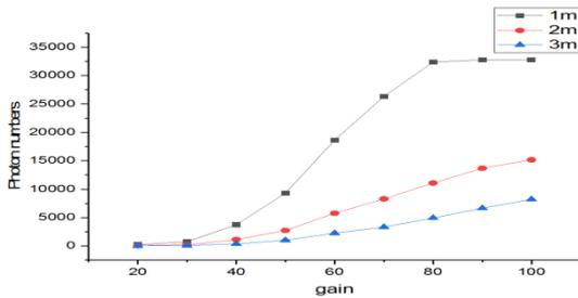
Figure 5: Uvolle equipment Corona measurement graph by distance (1, 2, 3m)
