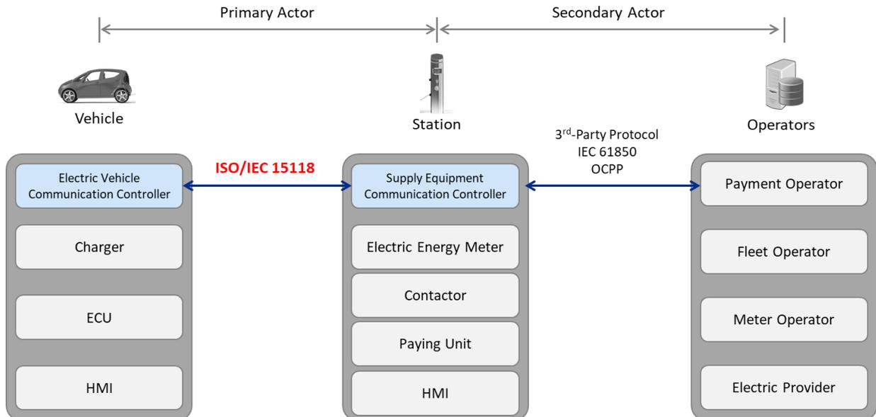
Figure 1: Scope of ISO / IEC 15118 Electric Vehicle Infrastructure Standard
