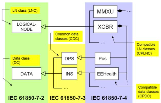
**Figure 3:** Data stack and Data representation method of IEC 61850
