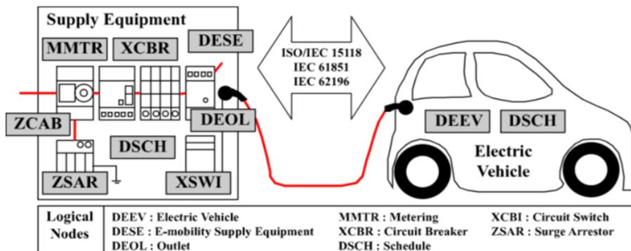
Figure 5: Linkage model of electric vehicle data in IEC 61850-90-8
