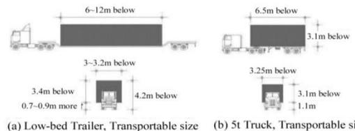
Figure 6: The size of the movable module unit according to the transportation equipment
