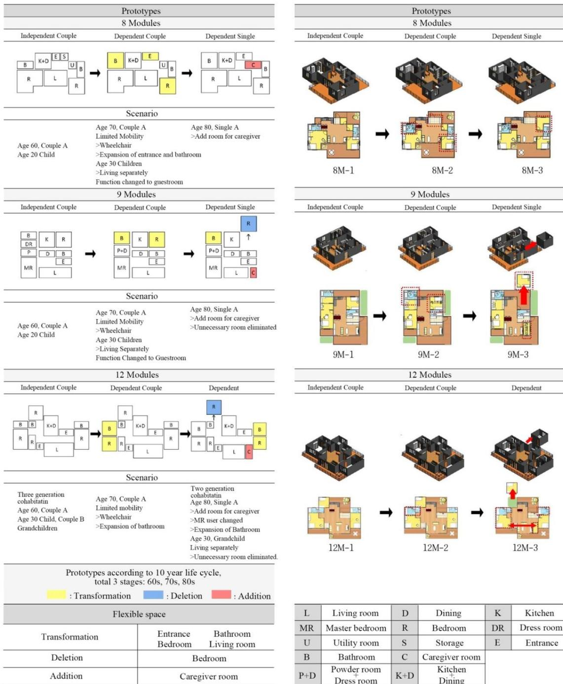
Figure 10: Flexible modular housing prototypes according to the lifestyles and lifecycle of the elderly
