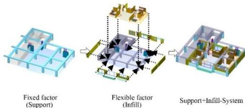
Figure 7: Flexible housing elements
