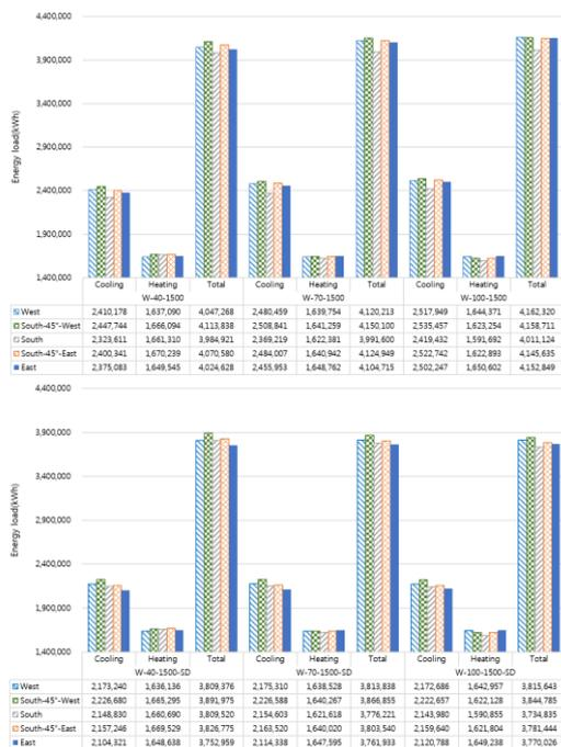
Figure 7: Energy load within double-skin facade (air gap 1500mm)
