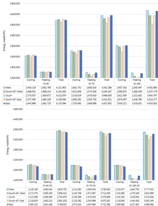
**Figure 2: Energy load without the double-skin facade**
