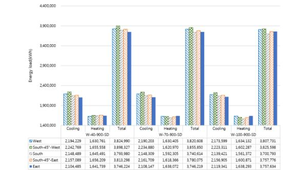
Figure 5: Energy load within double-skin facade (air gap 900mm)
