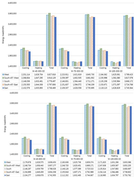
Figure 4: Energy load within double-skin facade (air gap 600mm)
