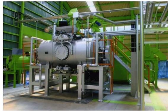
Fig.6: High-temperature high-pressure hydrolysis carbonization equipment (AandA Ltd.)
