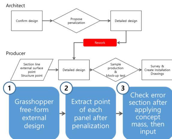
Fig 3: Flow chart of 1st alternative
