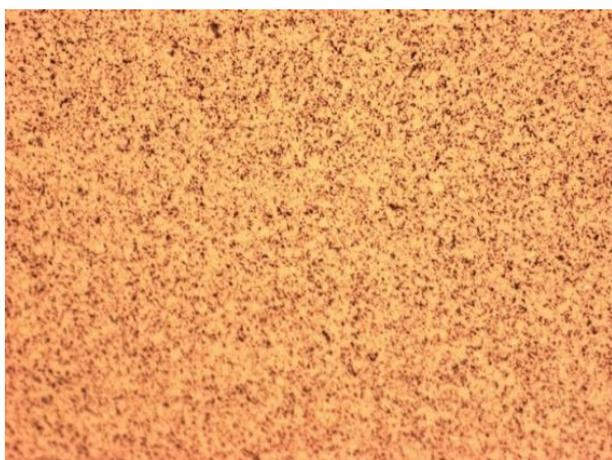
Figure 8: PCD Surface after WEDM Process (x200)
