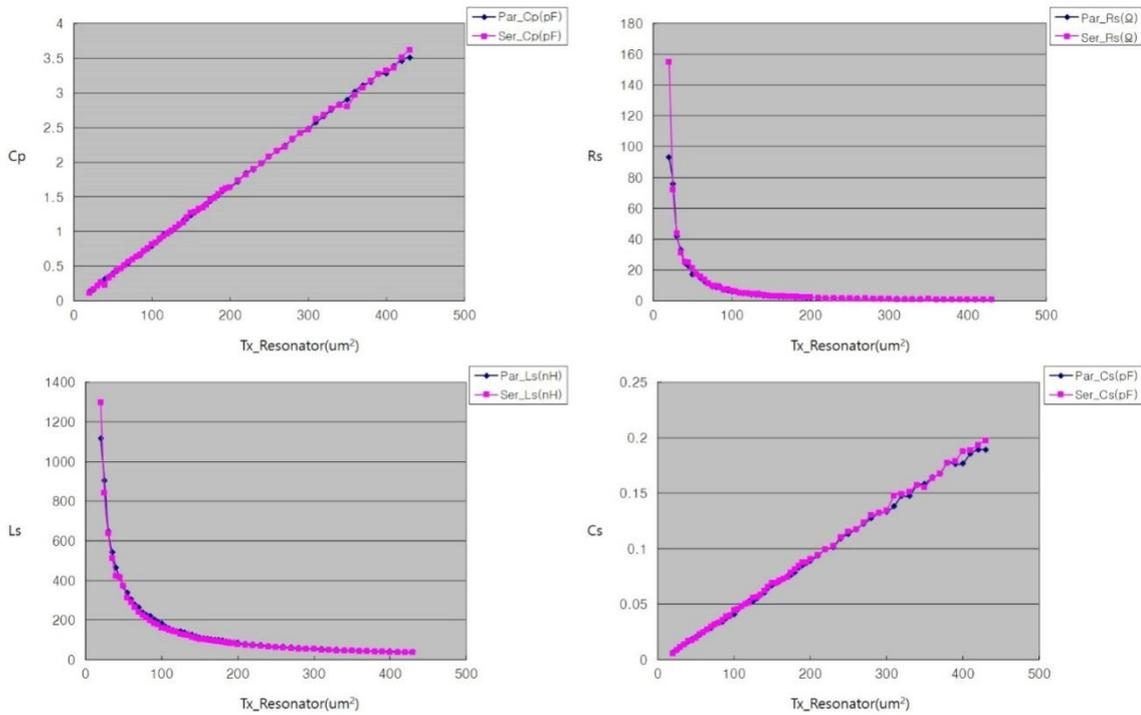
Figure 4.: MBVD Parameters for Ser.&Par. resonators
