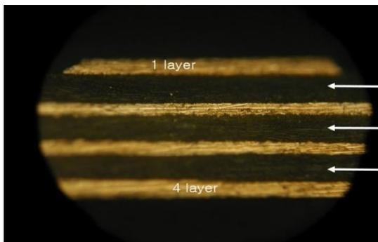
Figure 12.: Structure diagram for PCB multilayer
