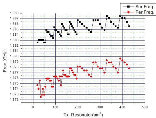
Figure 3.: Frequency deviation by resonator size
