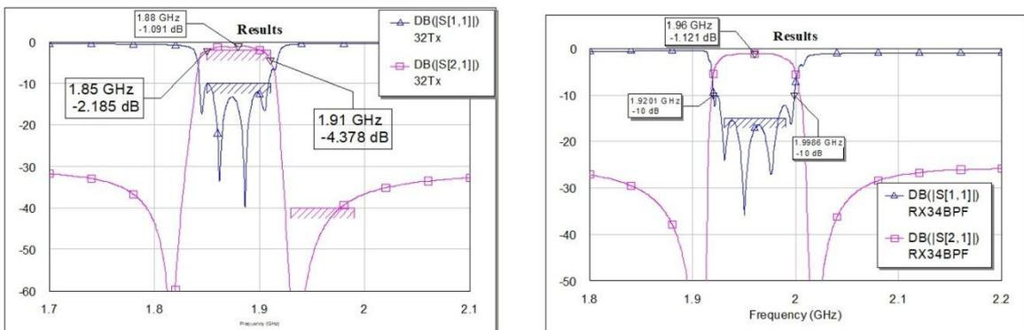
Figure 6.: Results of S11 and S21 for Tx, Rx Filter
