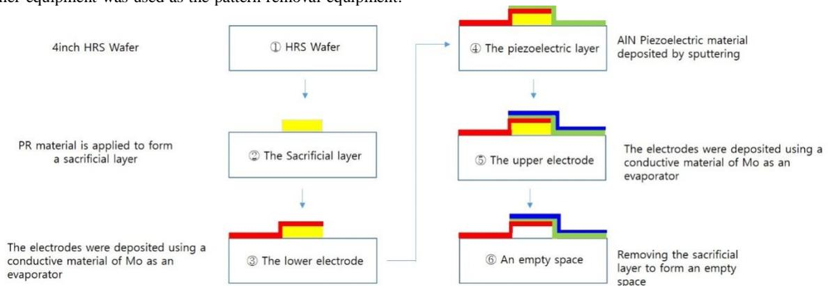
Figure 2.: Process for fabricated FBAR
