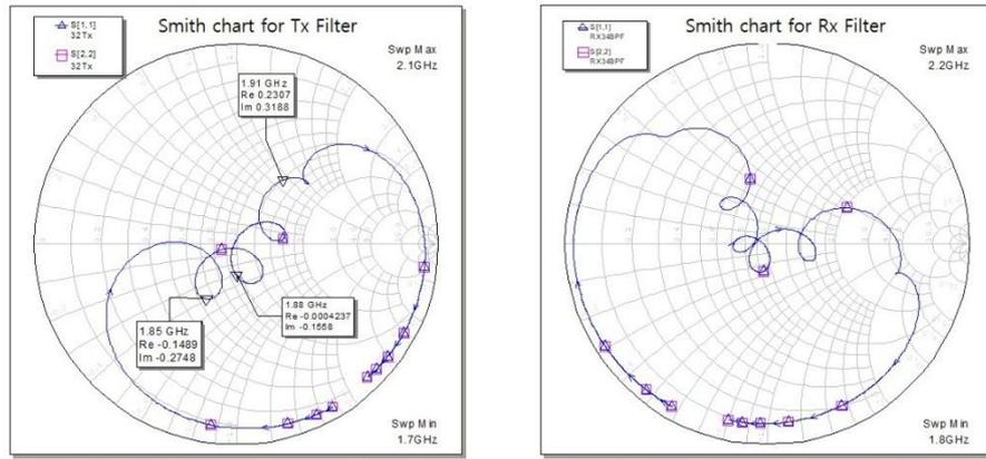
Figure 7: Smith chart of S11 and S21 for Tx, Rx Filter
