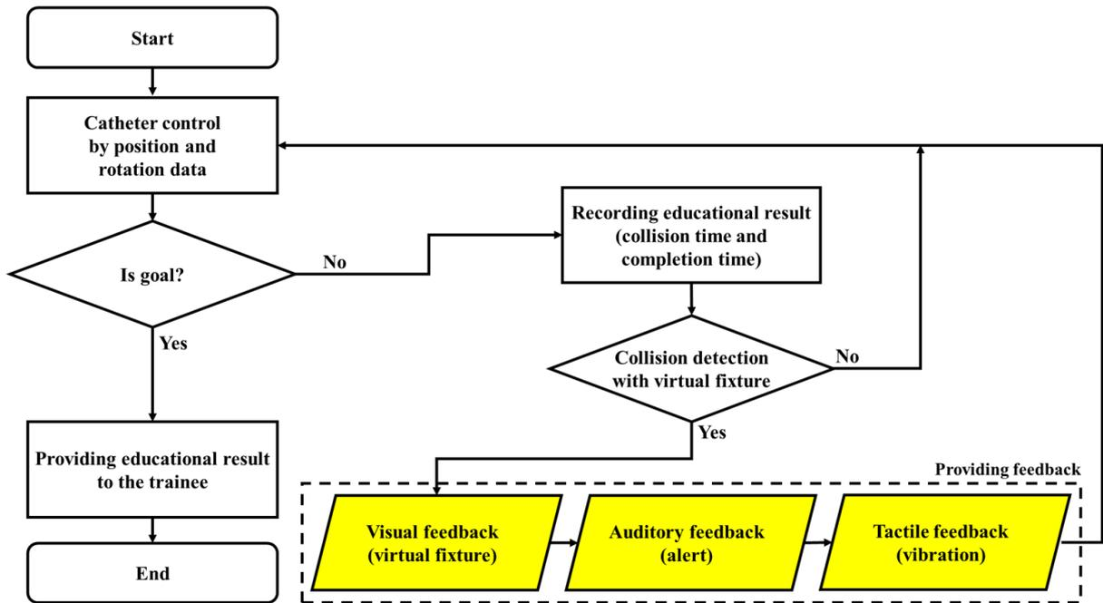
Fig. 3: Flowchart providing feedback effects of EpiduroSIM™
