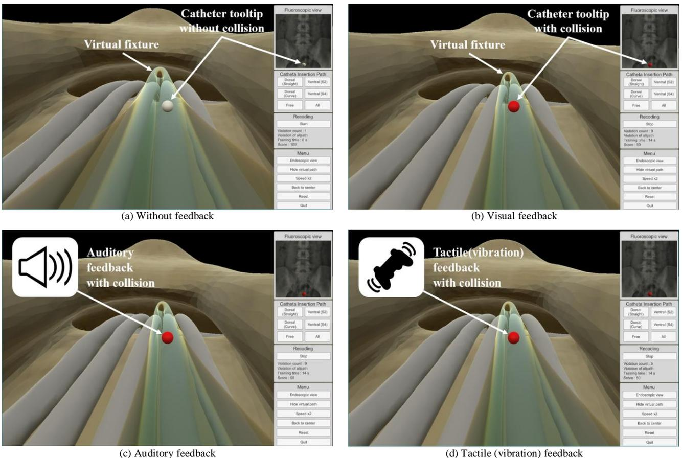
Fig. 4: Feedback effects applied to EpiduroSIM™
