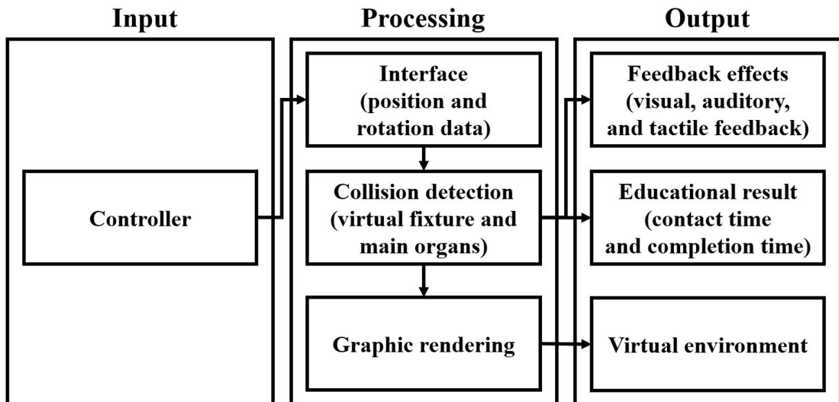
Fig. 1: Blockdiagram of EpiduroSIM™
