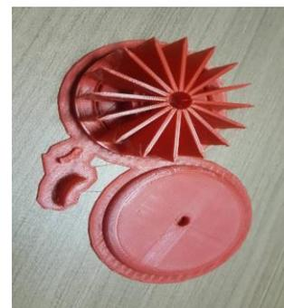
Fig 5: Prototype structure of the airflow sensor.
