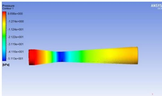
**Fig. 6:** Pressure contour for nozzle with converging angle,  $\theta_1 = 18^\circ$  and inlet hole position,  $X = 59.5$  mm
