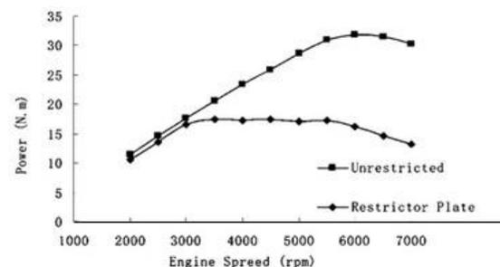
Fig. 1: Effect of air restrictor on the engine power [2]
