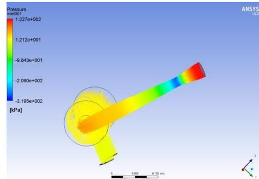
**Fig. 8:** Pressure contour for Design 1
