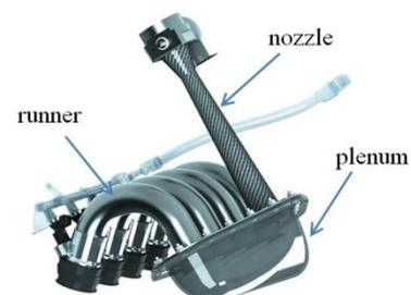
Fig. 2: Example of Formula SAE car engine restrictor system [3]
