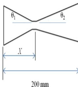
**Fig. 4:** Converging and diverging nozzle parameters
