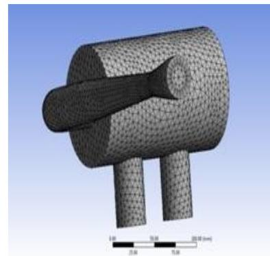
**Fig. 5:** CFD model of Design 1
