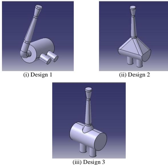
**Fig. 3:** Different types of restrictor design (i) Design 1, (ii) Design 2 and (iii) Design 3
