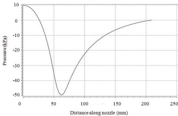
**Fig. 7:** Pressure vs distance along nozzle axis with converging angle,  $\theta_1 = 18^\circ$  and inlet hole position,  $X = 59.5$  mm
