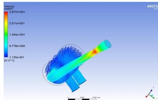
**Fig. 9:** Velocity contour for Design 1
