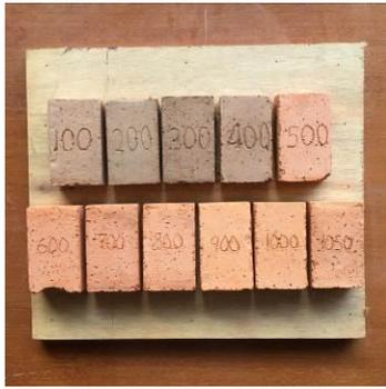
Fig. 3: PKS brick after fired at different temperature
