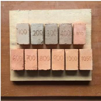
Fig. 4: EFB brick after fired at different temperature
