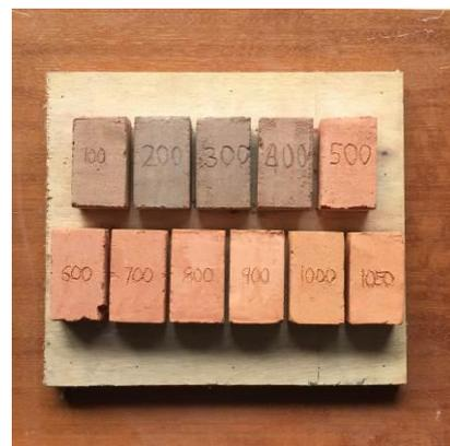
Fig. 2: Control brick after fired at different temperature
