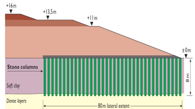
Fig. 1: Typical cross-section of the embankment in Boulevard in Putrajaya, Malaysia [1]
