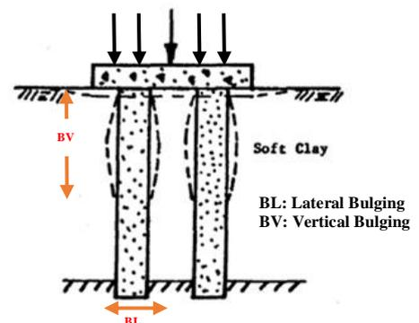
Fig. 9: Bulging failure on small columns group
