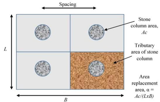
Fig. 2: Geometrical detail of LECA column
