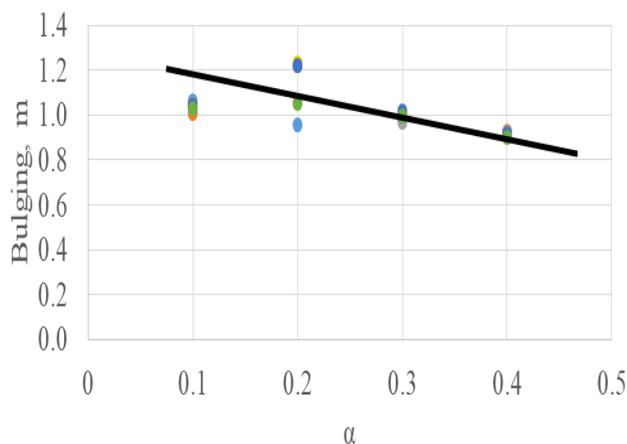
**Fig. 10:** Bulging failure for varies area replacement area
