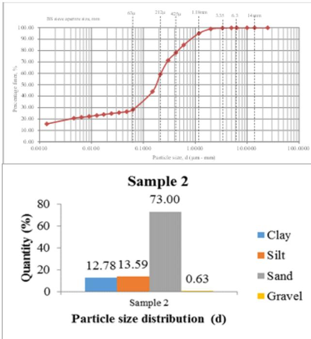
Fig. 11: Particle size distribution for sample 2
