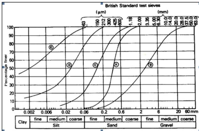
Fig. 2: Particle size distribution based on British standards [3]
