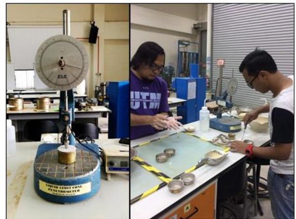
Fig. 8: Liquid limit (left) and plastic limit (right) test
