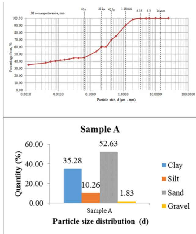
Fig. 12: Particle size distribution for sample A
