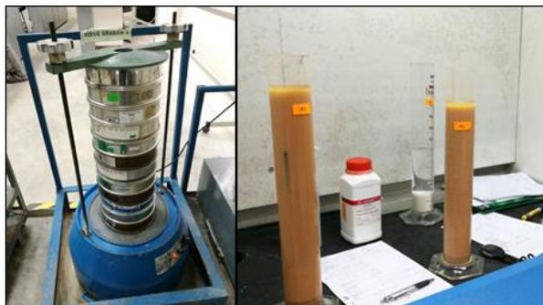
Fig. 7: Dry (left) and wet (right) sieve in progress
