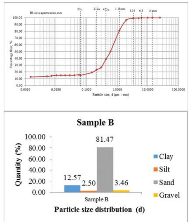
Fig. 13: Particle size distribution for sample B
