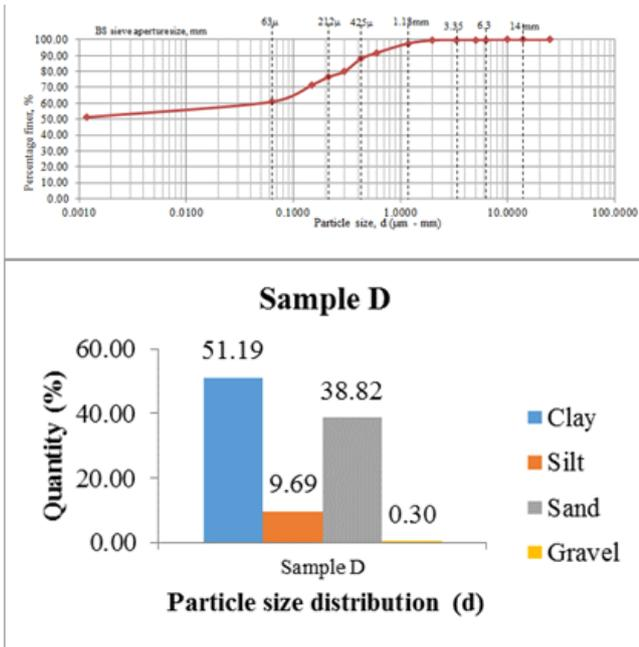
Fig. 15: Particle size distribution for sample D
