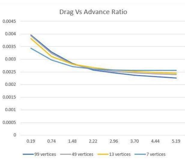
Fig. 7: Drag Versus Advance Ratio
