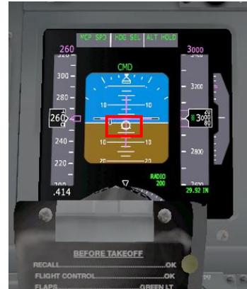
Fig 27: An aircraft cruising in X-Plane indicating with flightpath indicator (white circle in red square) lies on artificial horizon indicator. And the Vertical Speed Indicator is zero.
