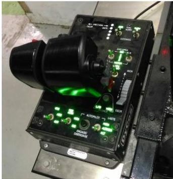
Fig. 24: Thrustmaster Hotas Warthog Engine Controller
