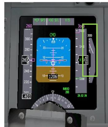
Fig 29: An aircraft climbing in X-Plane indicated with Vertical Speed Indicator shows positive values (green square).
