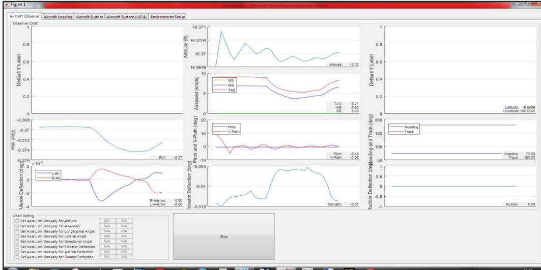
Fig. 17: Aircraft observer window in plotting received data
