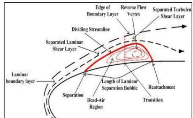
Fig. 1: Laminar Separation Bubble [1]
