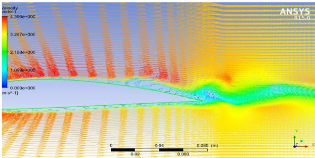
Fig. 10: Velocity vector for NACA 4415
