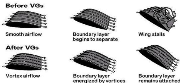
Fig. 3: Effect of vortex generators [3]
