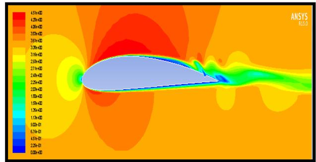
Fig. 13: velocity contour at 0 degree AOA with inward dimple
