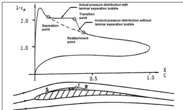
Fig. 2: Pressure distribution over airfoil with LSB [2]
