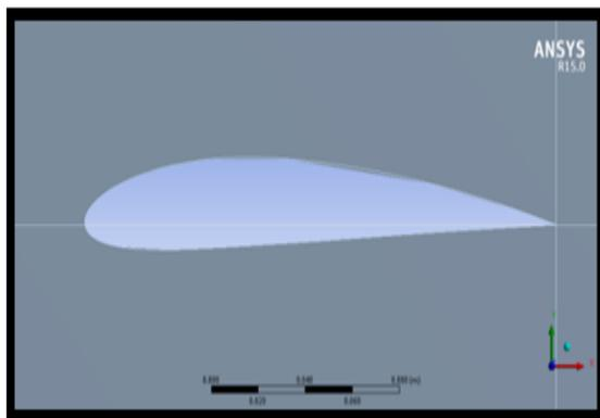
Fig. 6: Geometry of NACA 4415 aerofoil created in ANSYS
