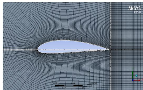
Fig. 9: Structured mesh for the entire domain
