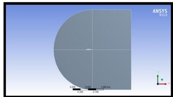
Fig. 8: Domain around the aerofoil for NACA 4415
