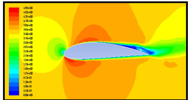
Fig. 14: velocity contour at 0 degree AOA with outward dimple
