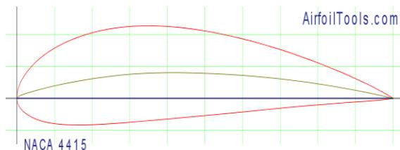
Fig. 5: NACA 4415 airfoil section [5]
