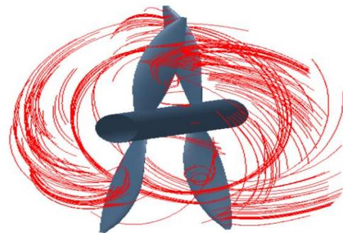
Fig. 20: The streamline that shown the swirlflow and a little of circulation flow when the stream through to the rotation of contra-propeller in the duct.
