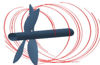
Fig. 21: Flow visualization of tip swirl flow at the ducted contra rotating (isometric view)
