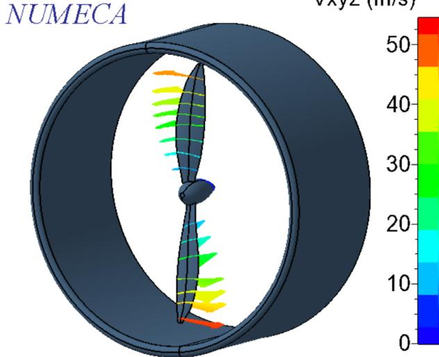
Fig. 16: Velocity distribution along the spanwise propeller
