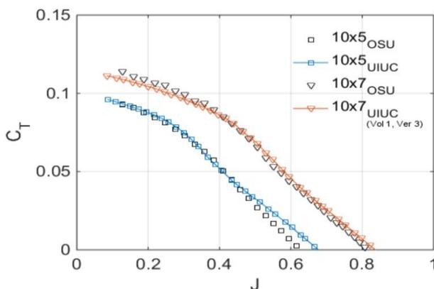
Fig. 12: UIUC propeller data for 10x5 and 10x7 thin electric propeller
