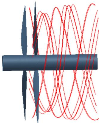
Fig. 22: Flow visualization of tip swirl flow at the ducted contra rotating (Side view)
