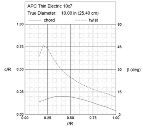
Fig. 3: Single propeller geometry: APC thin electric 10x7
