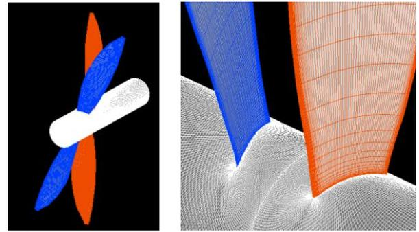
Fig. 8: the three dimensionaol of structured mesh contra rotating propeller
