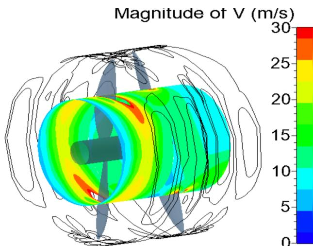
Fig. 23: Velocity contour of the contra rotating propeller domain shows the velocity change through the duct.
