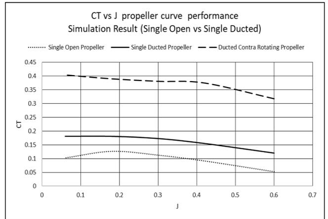
Fig. 18: Coefficient of thrust (CT) comparison of each cases
