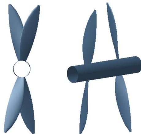
Fig. 19: Geometry of the contra rotating propeller, the same propeller is just stacking without any modification in pitch blade.
