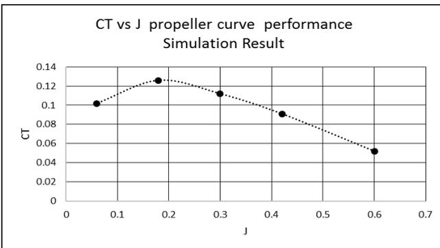
Fig. 11: CT (Thrusts Coefficient) versus J (advance ratio) based on the isolated propeller CFD
