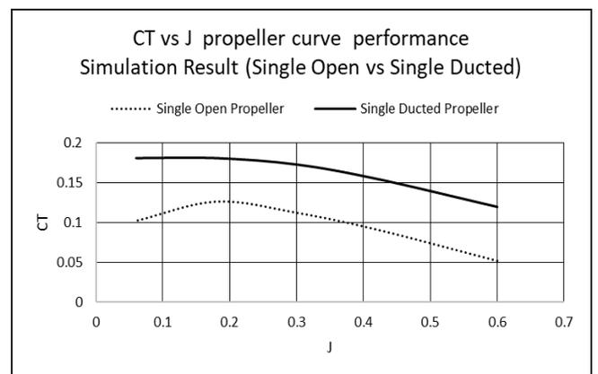
Fig. 15: Comparison CT vs J curve between single open propeller and single ducted propeller
