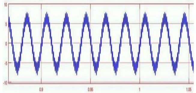
Fig.9: Voltage output of inverter after current controller implementation
