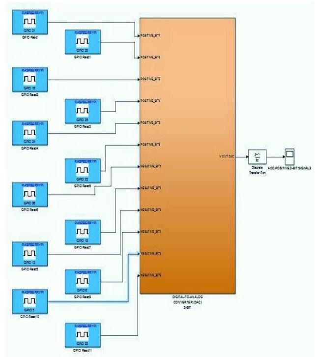
Fig. 4: DAC 3-Bit system
