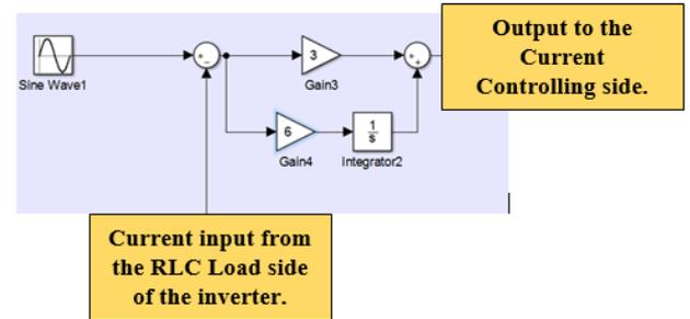
Fig.5: PI Controller block in MATLAB-Simulink
