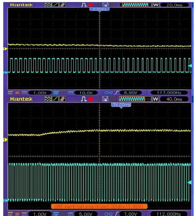
Fig.11: Output of the PWM signals to the inverter with current control
