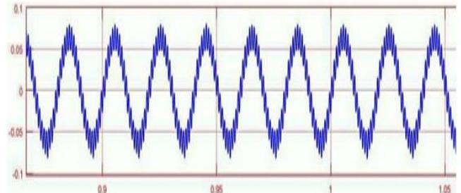
Fig.10: Current output of inverter after current controller implementation
