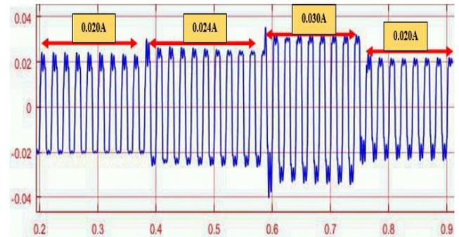
Fig.15: Output Current of inverter
