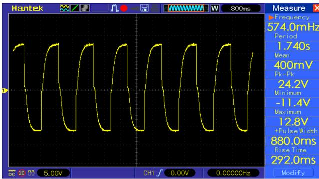
Fig 12: Output of the inverter with current control with filter
