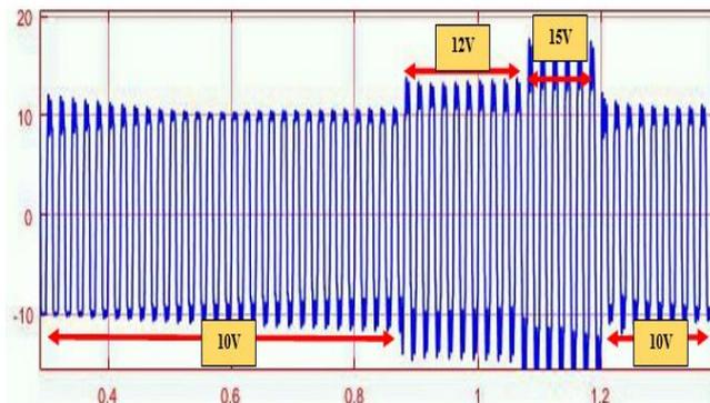
Fig.13: Output Voltage of inverter at varying inputs (filtered)
