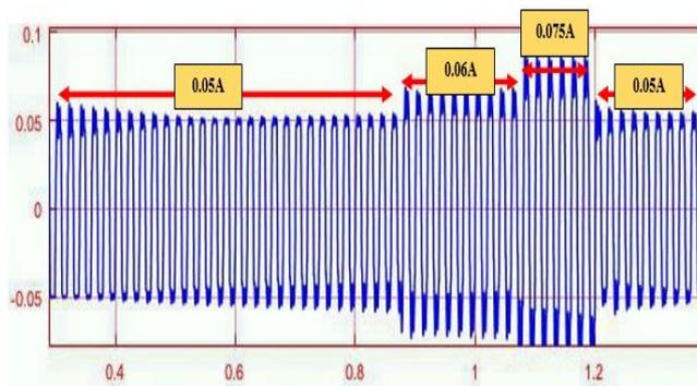
Fig.14: Output Current of inverter at varying inputs
