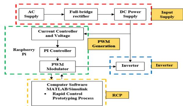
**Fig.1:** Block diagram for Rapid Control Prototyping of a single-phase back to back converter for a single phase network
