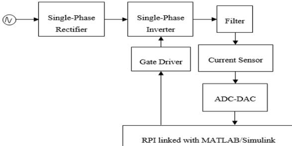
Fig. 2: Block diagram for RCP of a single-phase B2B
