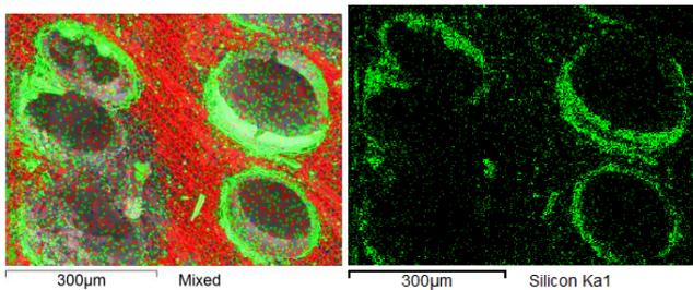
**Fig6:** Elemental mapping of silicon carbide (a) silicon (green) and carbon (red) element (b) silicon element (green)
