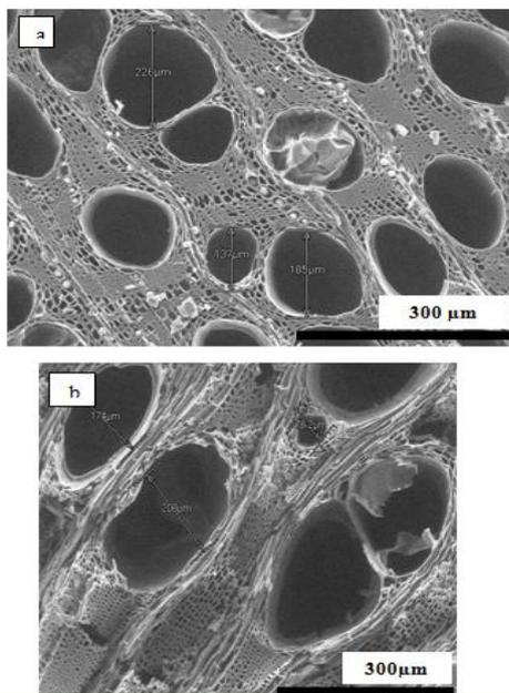
Fig 4: SEM micrograph of pyrolyzed wood from (a) Kapur and (b) dark red Meranti
