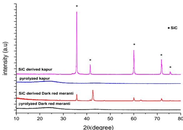
**Fig7:** XRD pattern of pyrolyzed carbon and resulting siC at 3 hours holding time
