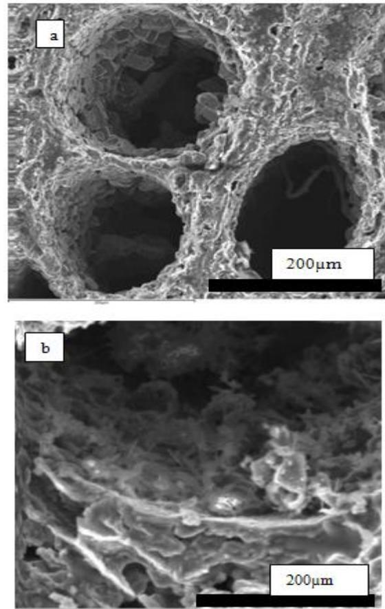
Fig. 5: SEM micrograph of SiC from (a) Kapur and (b) dark red Meranti
