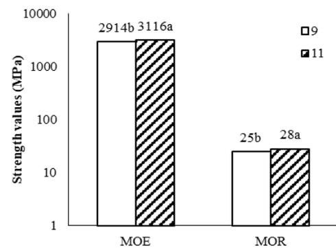
Fig. 5: Effects of resin content on modulus of elasticity (MOE) and modulus of rupture (MOR)
