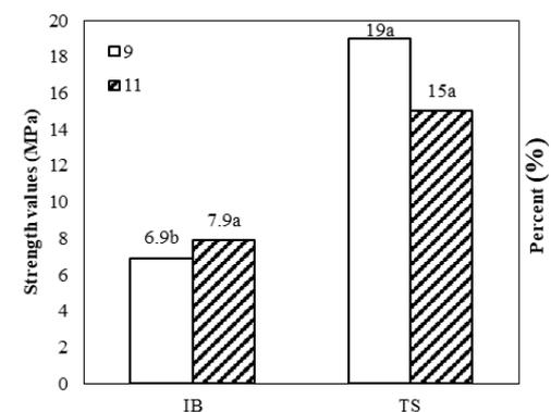
Fig. 6: Effects of resin content on internal bond strength (IB) and thickness swelling (TS)
