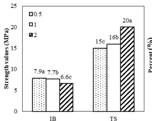
Fig. 2: Effects of particle size on internal bond strength (IB) and thickness swelling (TS)
