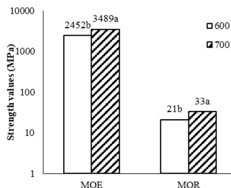
Fig. 3: Effects of board density on modulus of elasticity (MOE) and modulus of rupture (MOR)
