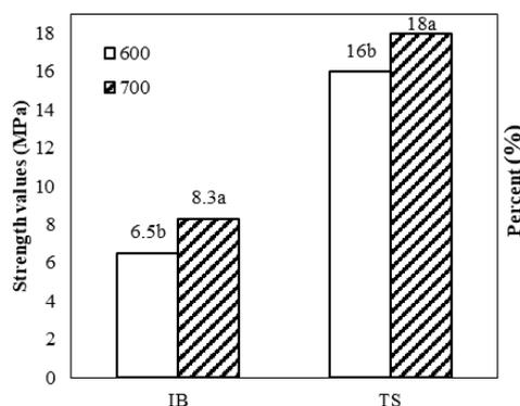
Fig. 4: Effects of board density on internal bond strength (IB) and thickness swelling (TS)
