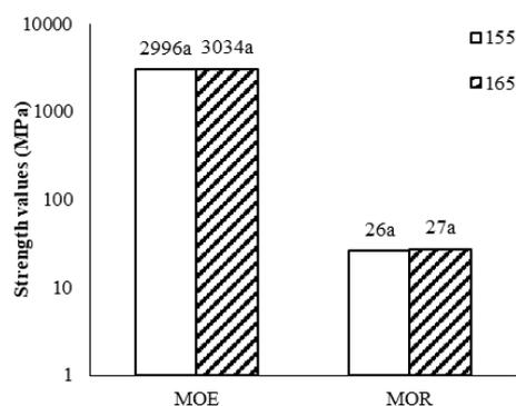
**Fig. 7:** Effects of hot press temperature on modulus of elasticity (MOE) and modulus of rupture (MOR)
