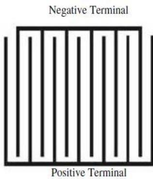
Fig. 3: Configuration of conventional planar interdigital sensor [4]
