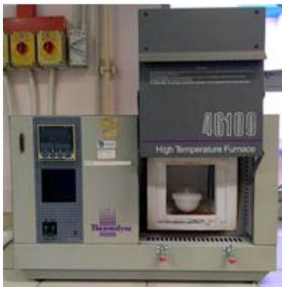
Fig 2: Calcination of as-synthesised powders
