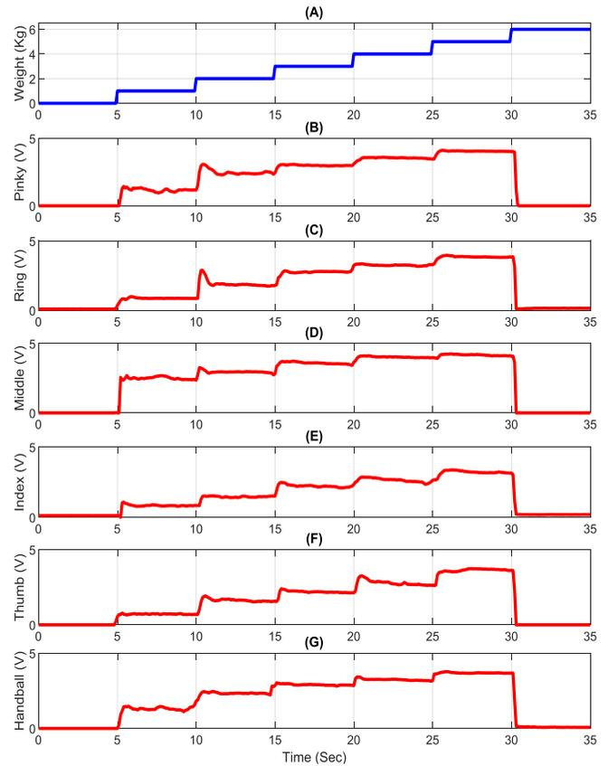
Fig. 9: The responses of the pressure sensors when the hanging weight increasing gradually
