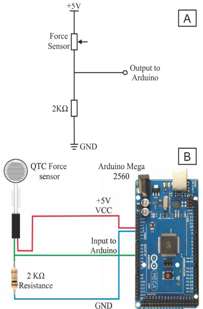
Fig. 4: Connecting the QTC pressure sensor with the Arduino Mega
