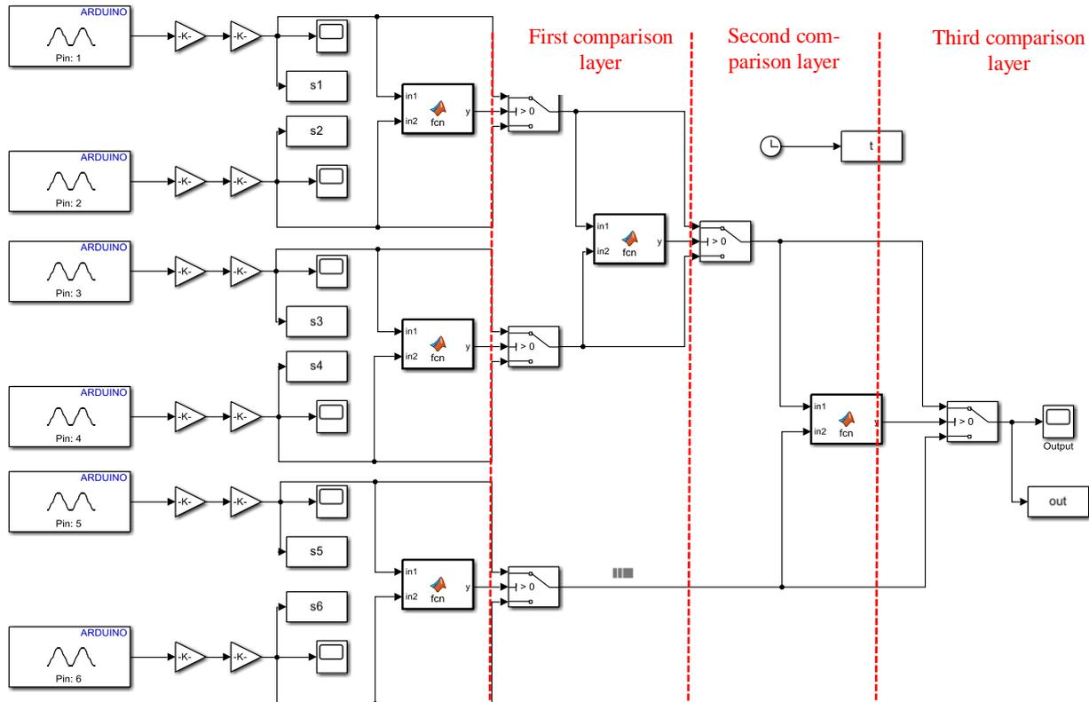
Fig. 5: Matlab/Simulink model of the tactile sensory glove
