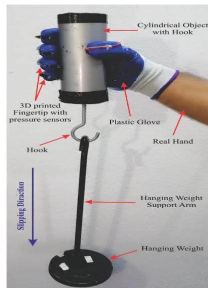
Fig. 7: Evaluation of slippage detection experiment
