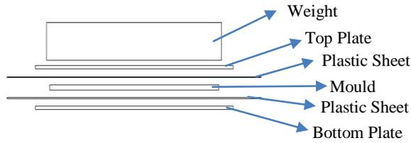
Fig. 2: Mould Arrangement
