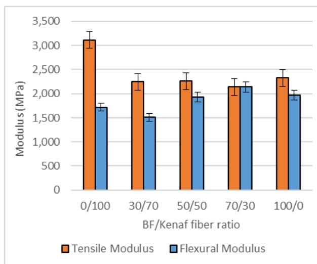
Fig. 11: Tensile and Flexural Modulus of BF/Kenaf/Polyester composites
