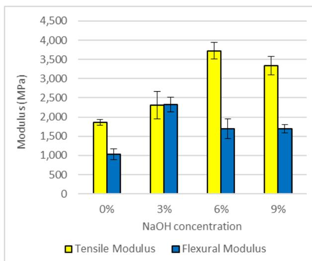
Fig. 5: Tensile and Flexural Modulus of BF/epoxy composites
