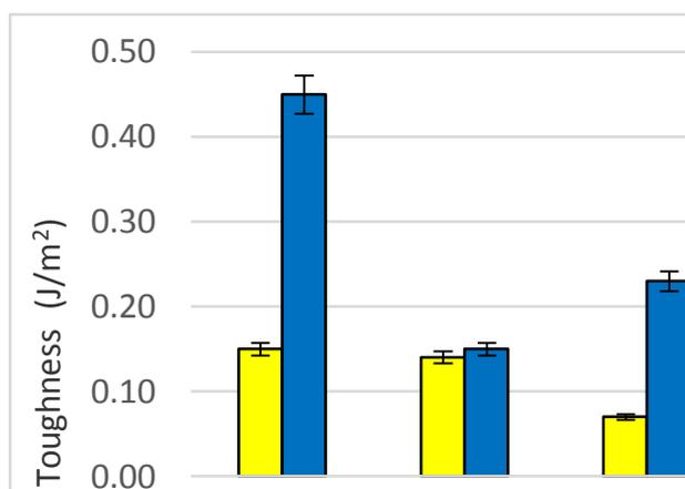
Fig. 6: Tensile and Flexural Toughness of BF/epoxy composite
