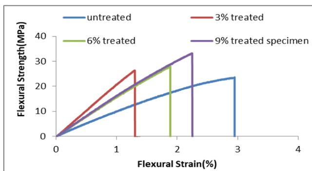
Fig. 3: Flexural stress-strain curves of BF/epoxy composites
