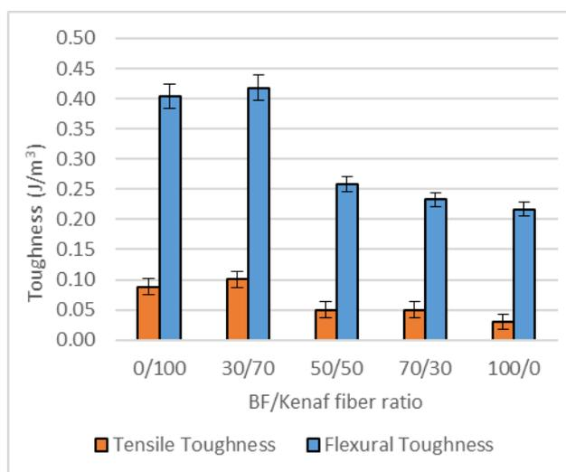
Fig. 12: Tensile and Flexural Toughness of BF/Kenaf/Polyester composites
