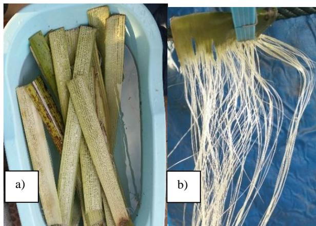
**Fig. 1:** a) Stack of Banana stem soak in water and b) extracting process of banana fiber
