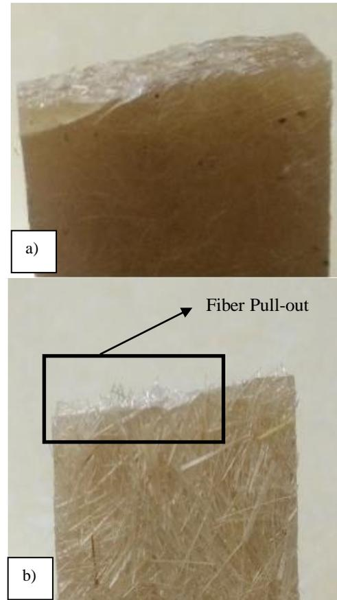
Fig. 10: a) Fractured Specimen a) 0/100 and b) 100/0 of BF/Kenaf/Polyester composites
