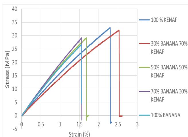
Fig. 7: Flexural Stress-strain Curves of BF/Kenaf/Polyester Composites
