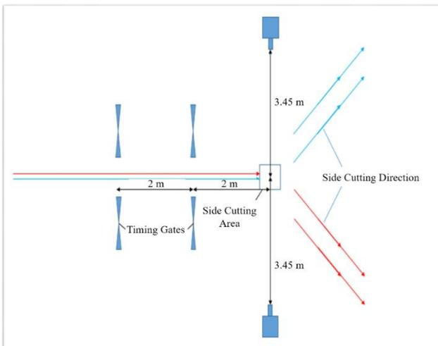
Figure 1: A Schematic Representation of the Side Cutting Task Layout.
